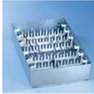
E 441/1 Insert 1/4 For use with upper and lower baskets in G 7831/G 7881/G 7891 • Mesh tray for micro instruments • 1.7 mm mesh spacing, solid sides, stackable • Internal sectioning with 6 adjustable partitions for easy arrangement of instruments • Can be autoclaved up to 121°C/134°C • H 60, W 183, D 284 mm
